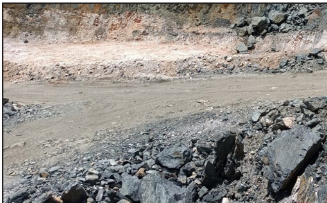
Figure 15: Morrua Tantalum mine showing the clear distinction between pegmatite (white) and barren basement rock (grey).
