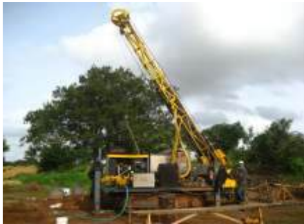
Fig-5 Diamond Core Drilling operation at Ganajur Main Prospect, Ganajur-Karajgi PL.
