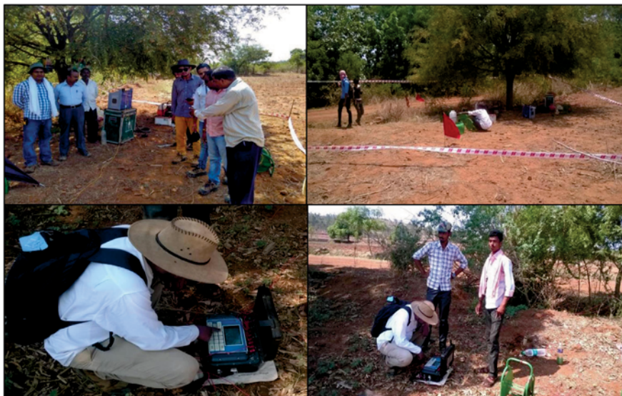
Fig-9: IP Survey Operation, Ganajur-Karajgi Cluster
